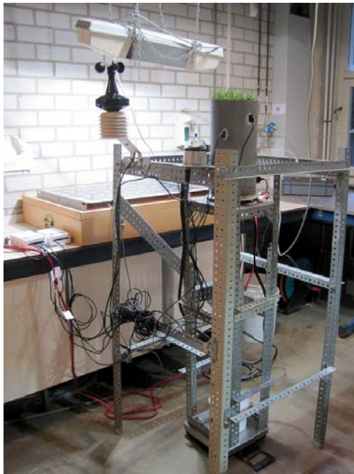
Figure 1 Lysimeter setup at UNESCO-IHE laboratory
