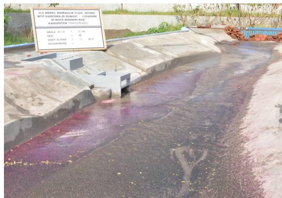
Figure 6 Combined cutting riverbank at upstream and downstream intake at +9.50 to +12.5 contour lines with addition of 2.5 m length of the intake situation
