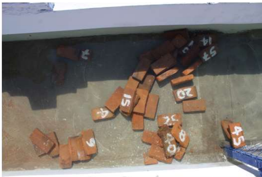
Figure 6 Result of an induced failure in the channel
