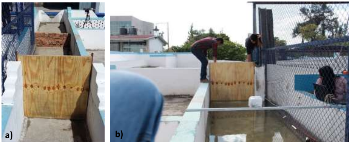
Figure 1 a) General view of the channel, tank storage area and flow-gate, b) Physical model operation
